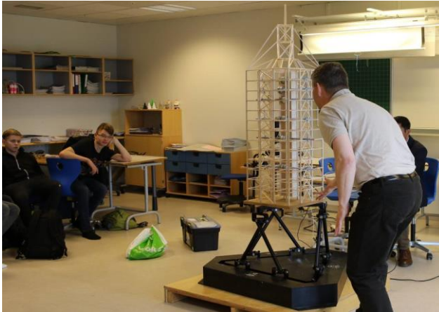
Figure 22. A balsa wood model of structural elements of a building mounted on a shaking table.
