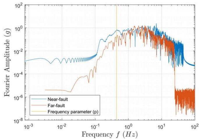
Figure 12: Fourier spectra of both records along with the Brimnes shelves frequency parameter.
