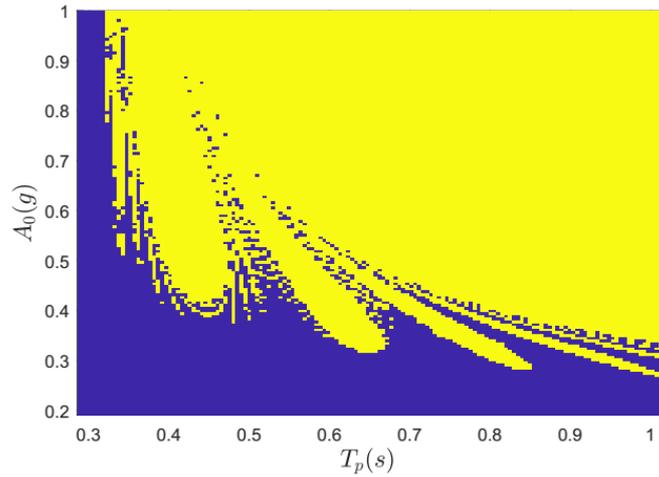
Figure 8: The overturning spectra of the Brimnes bookcase for single-sided rocking of rigid block.
