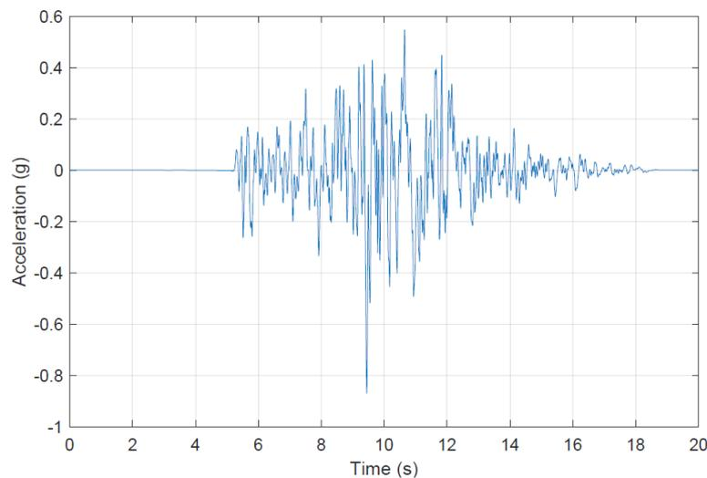
Figure 3. An example of simulated time series for hazard scenario at Selfoss ( $M_w \sim 6.5$  and fault distance  $\sim 5\text{km}$ ).
