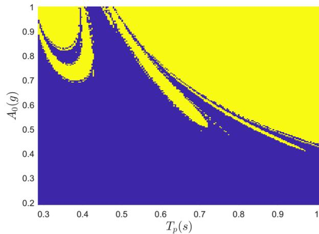
Figure 9: The overturning spectra of the Brimnes bookcase for two-sided rocking of rigid block.
