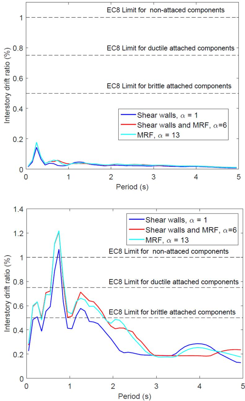
Figure 2. Drift spectra for Reykjavik (top) and Selfoss (bottom) scenarios, with 5% of critical damping.
