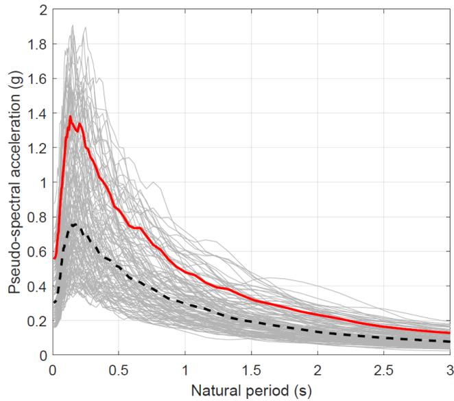
Figure 4. Response spectra of simulated ground motion for hazard scenario at Selfoss.
