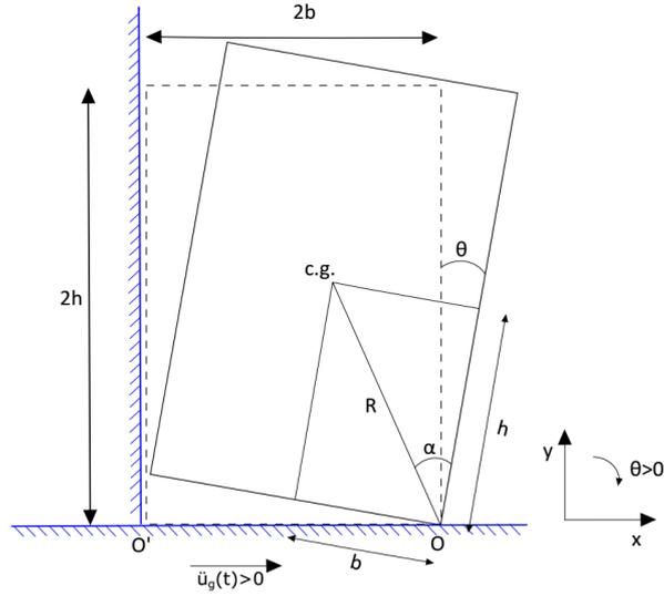
Figure 7 Schematic of a rocking block standing adjacent to a rigid wall.
