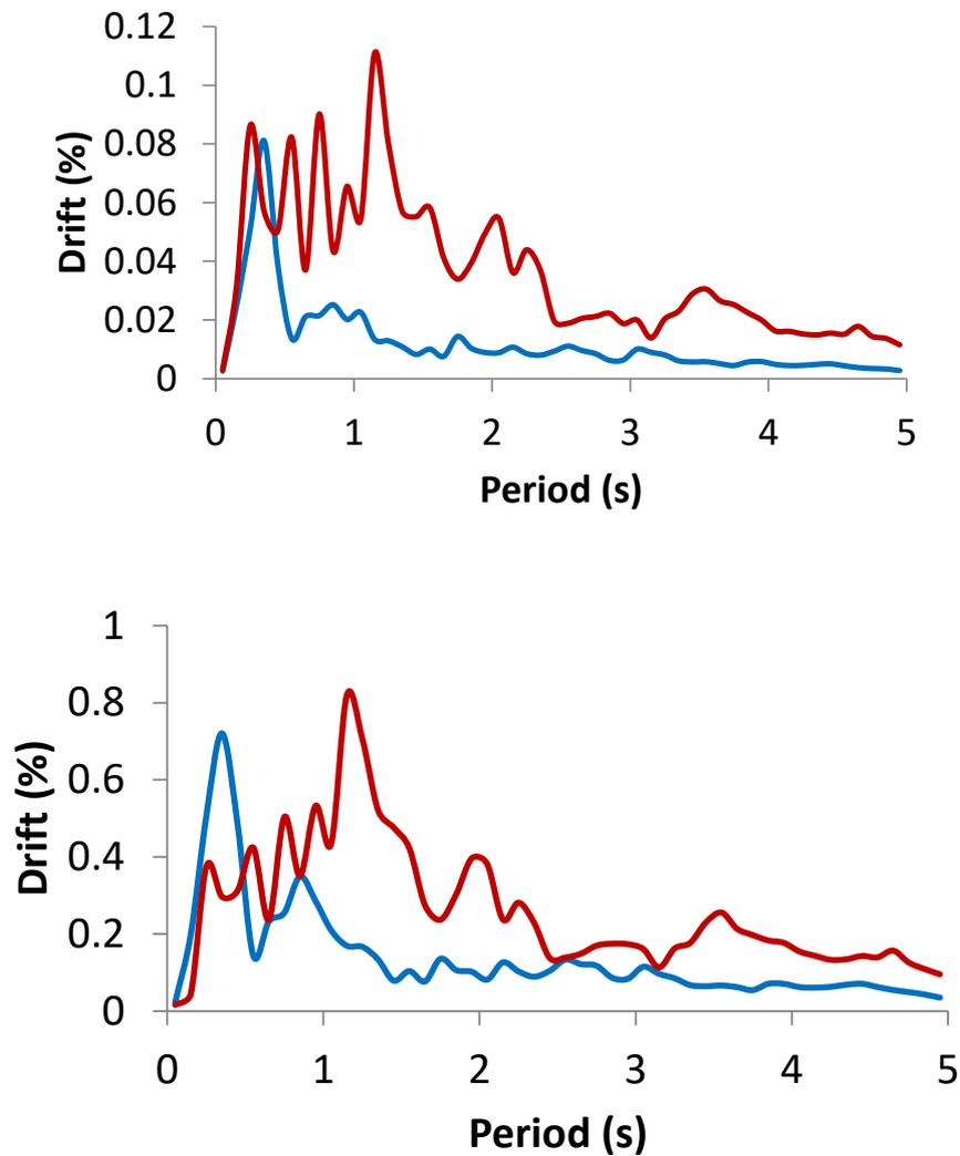
Figure 6. Maximum interstory drift spectra for two scenarios in hard rock and soft soil conditions in Zafferana.
