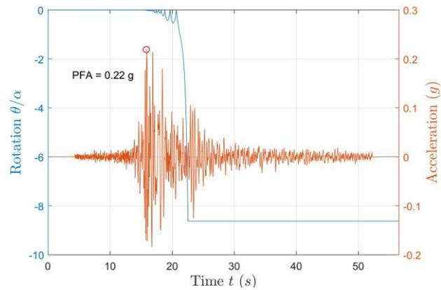
Figure 11: Numerical simulation of a one-sided rocking block excited by far-field ground motion
