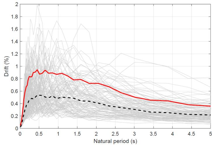
Figure 5. Drift spectra of simulated ground motions representing hazard scenario in Selfoss
