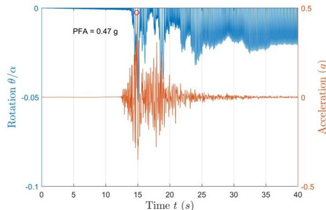
Figure 10: Numerical simulation of a one-sided rocking block excited by near-field ground motion.
